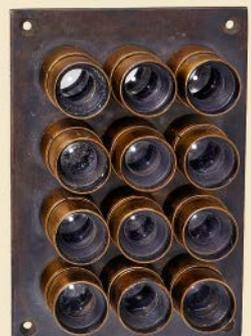
**French Multiplicator-Lens with 12 identic Petzval Lenses 4.5/50 mm, c. 1865**
